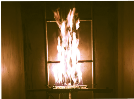
Heat measurement and smoke density during the flame propagation test -- EN50399 performed in a test cabin «CPR»
