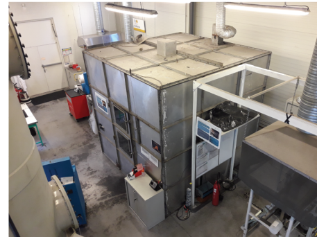
Smoke density measurement test -- EN61034-2 performed in a 27m3 test chamber.
