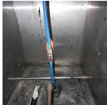
Flame propagation test on isolated cables -- EN 60332-1-2 performed with a 1kW burner. This is the only test to perform for the Euroclass E.
