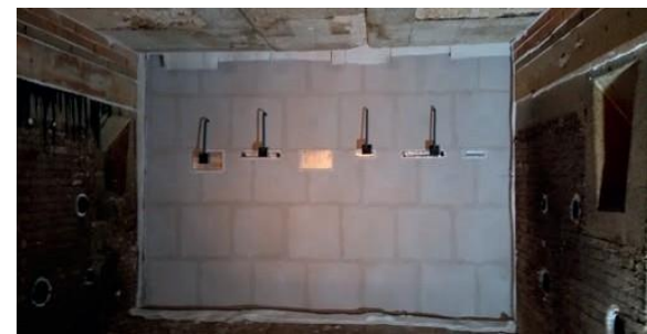
Fire exposed face of electronic enclosures for railway use before fire resistance test.
