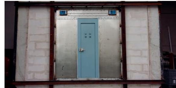
The side of a partition separating a driver's cab from a passenger compartment that is not exposed to fire before being tested for fire resistance.
